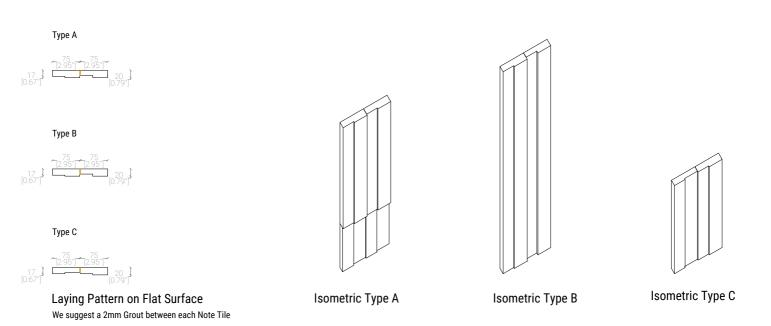
Please Note that Sierra Tile is assembled and composed by two or four different tiles jointed togheter.
